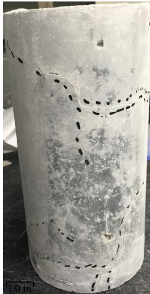
Figure 17: Cracking seen on samples stored in hot bath
