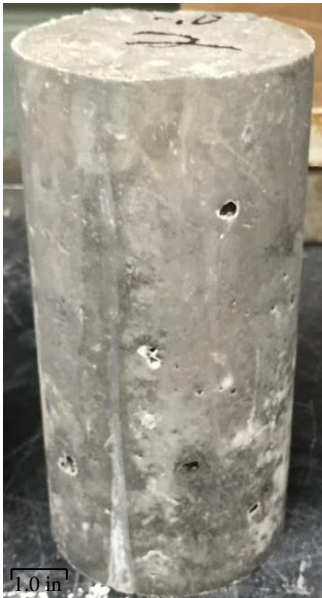
Figure 16: Sample stored in fog room displays no sign of cracking
