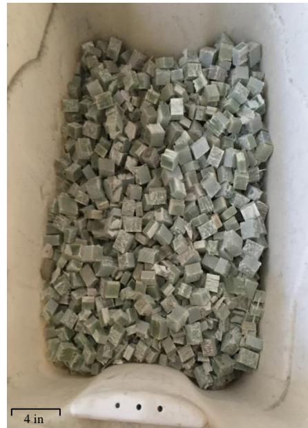
Figure 3: Composite aggregate created using manual process
