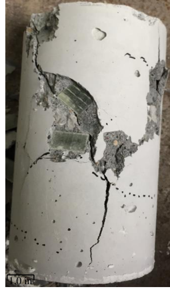
Figure 18: Compressive failure along cracking caused by curing
